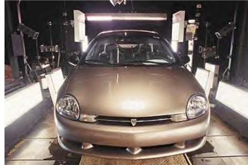
Paint film measurements/calculations are necessary in order to determine the maximum amount of product that can be removed in the de-nib and polishing process. By only removing quantities approved by OEM and Sikkens, can you insure paint film integrity.
